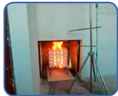
Ignition of the fire load made of 25kg of wood able to generate 250-300 kW.
