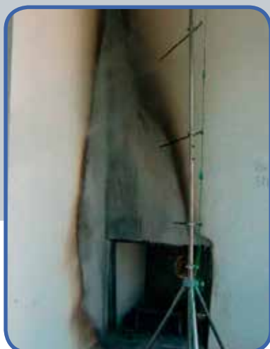
Turn-off phase at the end of 30' as required by procedure.
